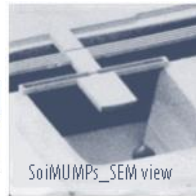
Deep reactive ion etching on silicon on insulator
