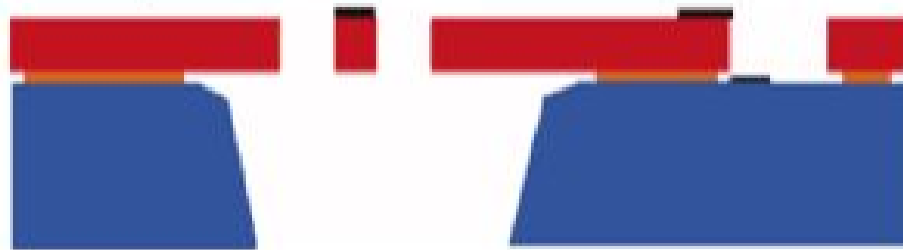
Figure 1: cross section view of the SOIMUMPS surface micromachining technology
